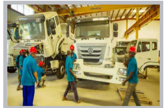
SINOTRUCK FZE assembles different sizes of Dump Trucks for Nigeria market
